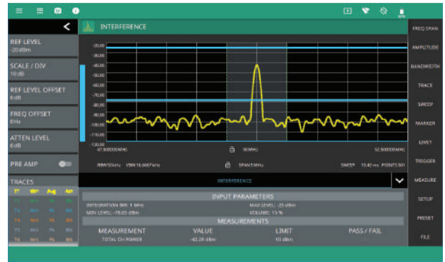
Interference Finder Option 24 Provides Fast Audio Tone Response to Changing Interference Levels
