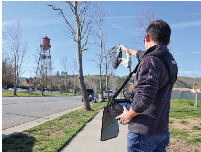
A Directional Antenna Coupled to the Interference Hunter MA2700A Provides Rapid Geolocation of RF Sources
