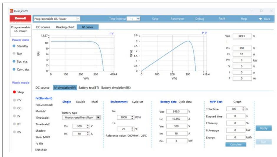
Figure 4-10 IV simulation function
