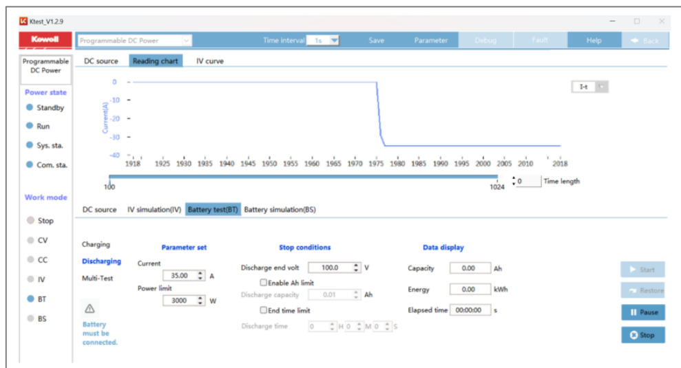
Figure 4-8 Static discharging mode
