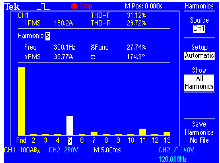
Conduct harmonic distortion measurements with TPS2PWR1 software.
