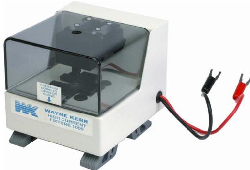
1009 Fixture enables 50 A to be applied to an SMD inductor
