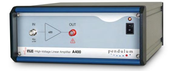
HIGH VOLTAGEFIXED GAINBROADBAND±200V20xDC to ca 500 kHz150mAFULL SCALELOW OUTPUT IMPEDANCEHIGH SLEW RATE<0.1 Ω</td>400 V/µs
