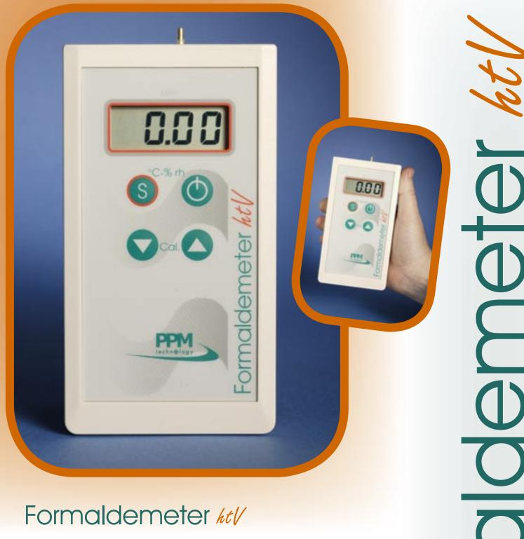
The latest 3-parameter instrument from PPM Technology directly measures airborne formaldehyde concentrations as well as ambient temperature and humidity levels.
