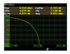
Noise-Like signals are analyzed statistically. The average power in this CCDF representation serves as a reference, while the graph shows the distribution of lower power levels.
