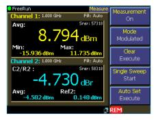
Large numeric displays allow comfortable measurement control.
