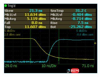
The Graphic Header feature of the 4541 / 4542 RF power meters allows displaying up to 10 user selectable parameters. Colors refer to the specific channel: yellow - ch1, blue ch-2.
