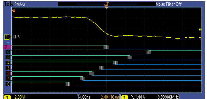
White edges indicate additional information is available by acquiring at a higher sample rate.
