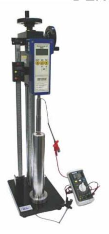
**DENSIPRESS** is an appliance to measure the bulk density of a powder as function of the applied pressure.
