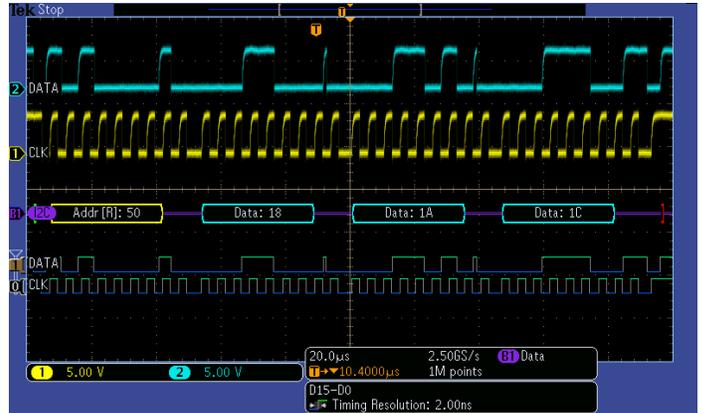
Triggering on a specific data packet going across an I<sup>2</sup>C bus. The yellow waveform is clock and the blue waveform is data. A bus waveform provides decoded packet content including Start, Address, Read/Write, Data, and Stop.
