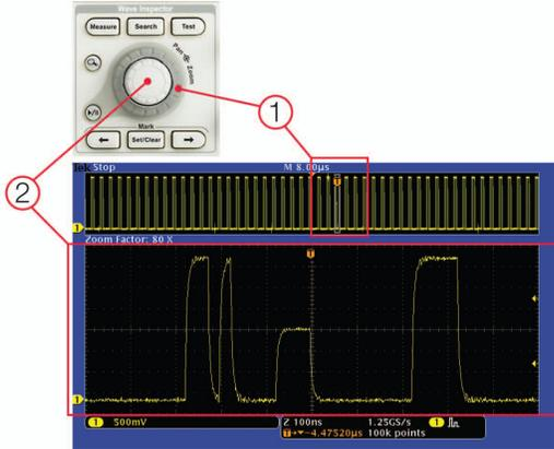
Wave Inspector controls provide unprecedented efficiency in viewing, navigating, and analyzing waveform data. Zip through your 5 Mpoint record by turning the outer pan control (1). Get from the beginning to end in seconds. See something of interest and want to see more details? Just turn the inner zoom control (2).
