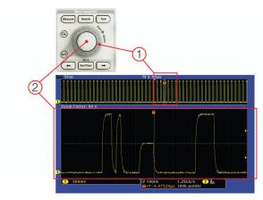
Wave Inspector controls provide unprecedented efficiency in viewing, navigating, and analyzing waveform data. Zip through your 5 Mpoint record by turning the outer pan control (1). Get from the beginning to end in seconds. See something of interest and want to see more details? Just turn the inner zoom control (2).
