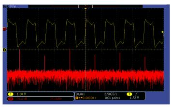
Analyze - FFT analysis of a pulsed signal. A comprehensive set of integrated analysis tools speeds verification of your design's performance.
