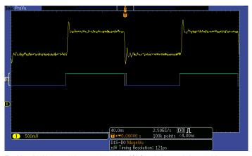
The MagniVu high-resolution record provides 121.2 ps timing resolution, enabling you to make critical timing measurements on your digital waveforms.
