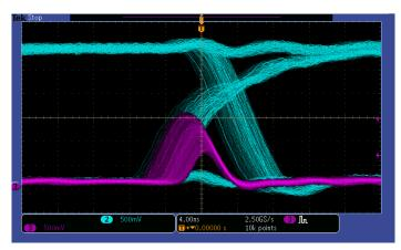
Digital phosphor technology enables greater than 50,000 wfm/s waveform capture rate and real-time intensity grading on the MSO/DPO3000 Series.
