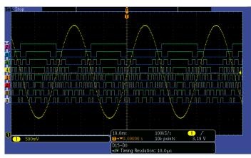
The MSO Series provides 16 integrated digital channels enabling you to view and analyze time-correlated analog and digital signals.
