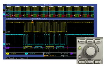
Search – I2C decode showing results from a Wave Inspector search for Address value 50. Wave Inspector controls provide unprecedented efficiency in viewing and navigating waveform data.
