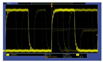
Discover – Fast waveform capture rate - over 50,000 wfm/s - maximizes the probability of capturing elusive glitches and other infrequent events.
