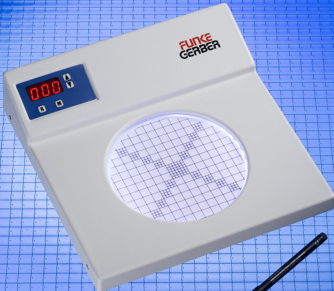
Counting Colonies is quick and simple. The counting impulses are activated by marking the colonies with a felt-tip pen. The counting impulse will be confirmed by an acoustical signal, which can be disabled. The pressure sensitivity for the count can be adjusted. Any ordinary felt-tip pen can be used for the marking.
