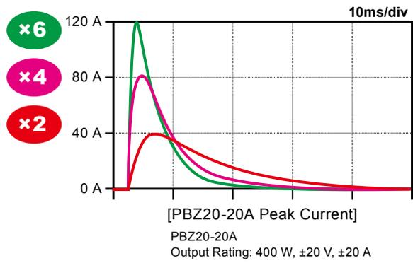
*Intelligent power supply providing arbitrary waveform generation and accurate power simulation!*
