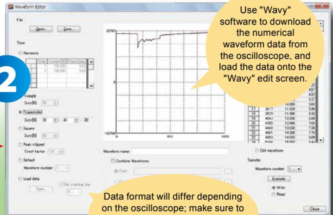
Use "Wavy" software to download the numerical waveform data from the oscilloscope, and load the data onto the "Wavy" edit screen.
