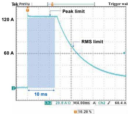
We recommend a maximum peak current output of up to 6 times the rating (5 times depending on output voltage) within a duration of 10ms (blue area on left). A minimum interval of at least 1 second is required between peak currents, as shorter intervals can cause hardware malfunction. The figure on the left shows the peak and rms current limits when the output is shorted.
