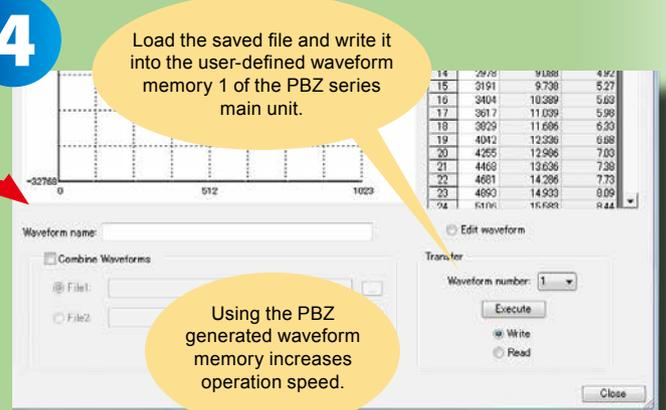
Load the saved file and write it into the user-defined waveform memory 1 of the PBZ series main unit.
