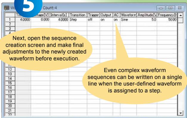
Next, open the sequence creation screen and make final adjustments to the newly created waveform before execution.
