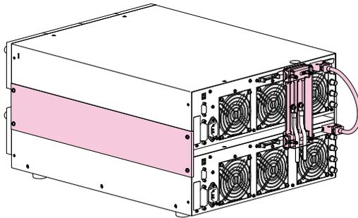
Parallel operation kit PK02-PBZ (For EIA inch size, option), PK03-PBZ (For JIS metric size, option) components
