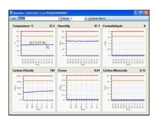
The PPMonitor software enables the data to be viewed graphically, produce reports and statistical data, run schedules as well as alarm functions and notifications for more effective and economical building management. It is possible to set up an Ethernet Access Point (EAP) to the wireless network which allows the wireless modules to be accessed from any location world-wide via the Internet provided the necessary internet address, firewalls and gateways are enabled on the local network.
