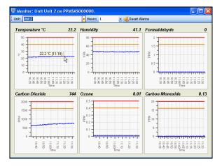
The PPMonitor software enables the data to be viewed graphically, produce reports and statistical data, run schedules as well as alarm functions and notifications for more effective and economical building management. It is possible to set up an Ethernet Access Point (EAP) to the wireless network which allows the wireless modules to be accessed from any location world-wide via the Internet provided the necessary internet address, firewalls and gateways are enabled on the local network.
