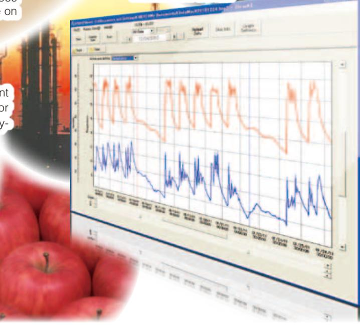
Use as a Voltage Logger to record pyranometer output for evaluating insulation.
