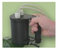
The instrument is supplied with three sets of light-emitting diodes and a PIN diode detector with 1 MHz/16-bit AD converter and software controlled gain and integration time.
