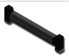
This new design is coil with a very stable and high quality ferrite core and tiny size (9 x 1.5 x 2 mm) and high sensitivity in low frequency range (20-40kHz). Those pieces are winding with thin copper wire up to12µm and its inductances range is 260-340 mH. Besides, it has good frequency and temperature behaviour and can be served with "custom" electrics characteristics according requirements of hearing aid devices manufacturers.
