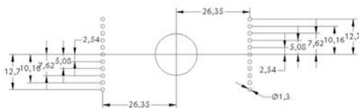
Recommended PCB layout
