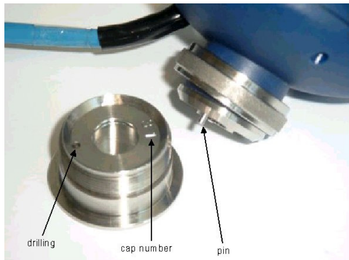
Fig. 1. Steel measuring cap. The drilling in the measuring cap is for holding a defined position between cap and pin in the head. The cap number in the measuring cap has to be concordant with the two last numbers of the head-ID.
