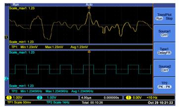
To find intermittent faults the TrendPlot  $^{\text{TM}}$  function can monitor measurements for long periods of time.
