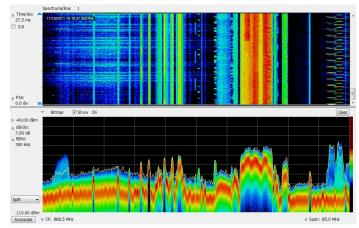
DPX Spectrograms provide gap-free spectral monitoring for up to days at a time. 60,000 traces can be recorded and reviewed, with resolution per line adjustable from 5.12  $\mu s$  to 6400 s.
