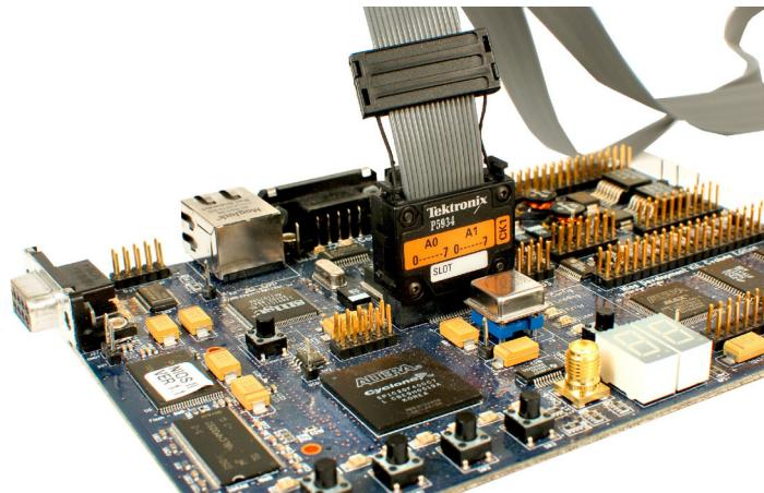
The P5934 is 34-channel micror probe with quick connect/disconnect and a positive latching mechanism to ensure a secure, reliable connection.
