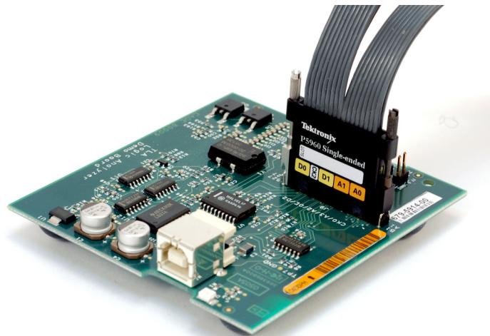
For applications where circuit board space is limited, the 34-channel high-density P5960 D-Max offers the smallest available footprint and a quick connection mechanism.
