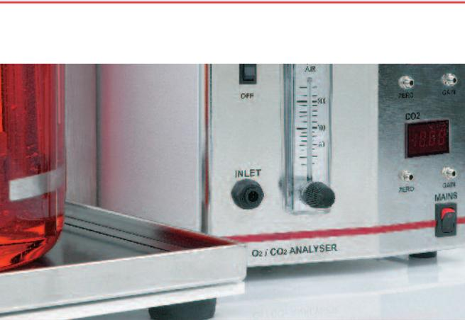
*The FerMac 368 Gas Analyser measures oxygen and carbon dioxide in exit gas, two important extra parameters which give the best indication of growth within a fermenter vessel. The Gas Analyser connects to the FerMac 360 Controller so that measurement can be logged and controlled by our software.*
