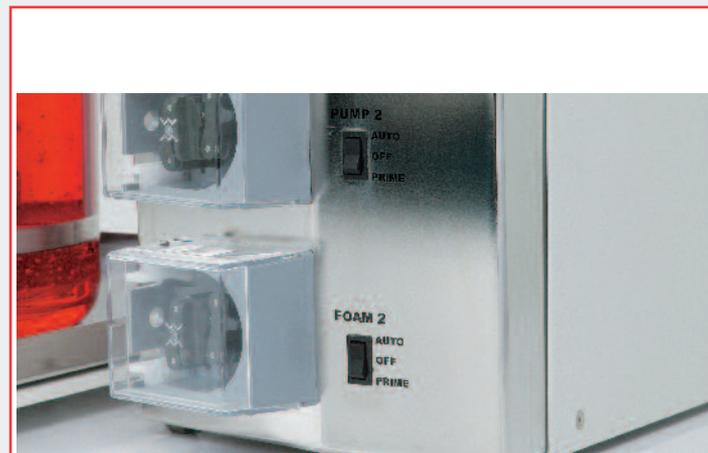
*The Electrolab Low Flow Rate Pump is specifically designed for bioprocess applications, providing a smooth flow of media with excellent reproducibility over extended periods of time.*
