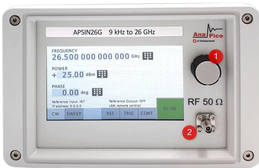
1. **Rotary Button** The rotary button is used to change the value selected on the screen.
