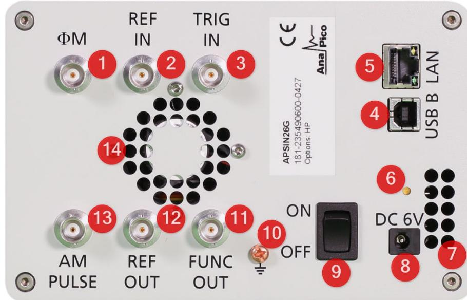
1. **ΦM** This BNC female Connector is the input for FM and PM.
