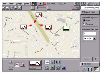
Locate interference with integrated mapping solution
