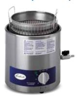
Endecotts' ultrasonic cleaner has been specially designed for cleaning test sieves and is also suitable for general laboratory use.
