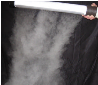
Optional Fog Curtain Wand to create a Curtain Fog to Visualize Airflow / Turbulence
