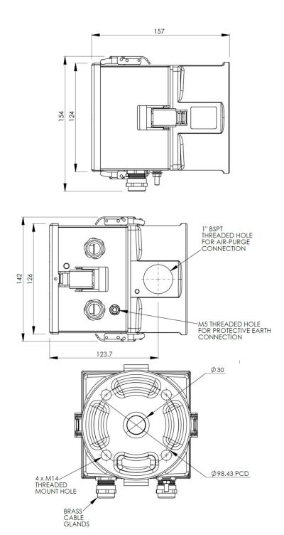
Note: The head shown is the RX head (two cable glands). The TX head (one cable gland) has exactly the same dimensions, but has one less cable gland.
