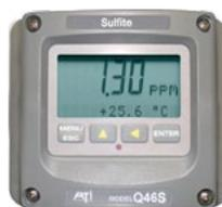
ATI's Model Q46S/66 Residual Sulfite Monitor provides the solution to dechlorination control in wastewater effluent. The sample stream is acidified which converts the sulfite ion into sulfur dioxide. The air-stripping system removes the sulfur dioxide from the solution and is measured with a gas-phase SO<sub>2</sub> sensor.
