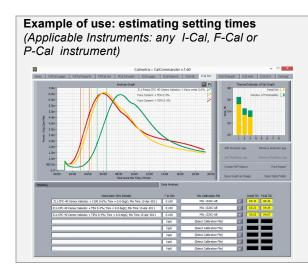
Isothermal calorimetry can be used to estimate setting times, as heat rates shown in the Power curve correlate with physical test data obtained applying a standard such as, for example, ASTM C403.
