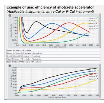
Shotcrete accelerators work through accelerated formation of calcium aluminate sulfate hydrates. The reactivity of the aluminate and sulfate phases in the binder used is of particular importance, both of which are visible in isothermal calorimetry, making it an excellent tool for optimizing admixtures for shotcrete as well as for the selection of binders for shotcrete.
