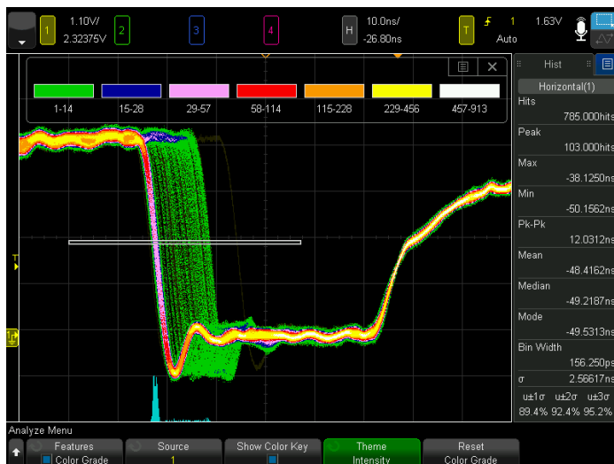
Figure 15. Color grade and histogram on a jittery clock edge.
