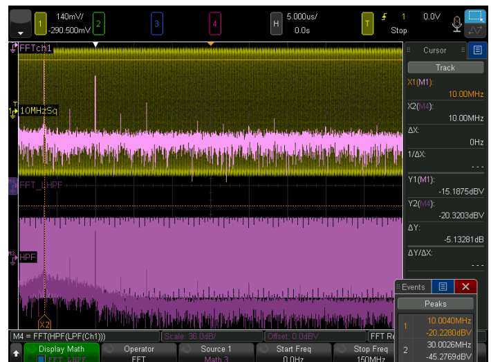
Figure 48. Four math functions used simultaneously (three turned on).
