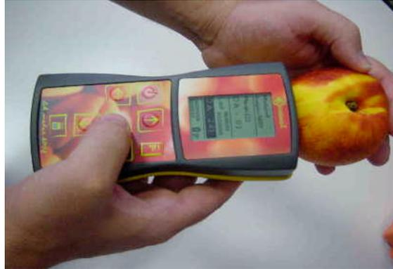
In fruit and vegetables establishing the optimal harvest time is a crucial issue, since fruit shelf-life potential and quality are closely related to the ripening stage at harvest. The DA Meter is a very promising tool both for practical and scientific applications, since it allows to monitor on-tree fruit ripening (as well on the same fruit), to establish accurately the optimal harvest time and it can be used in cool store to establish maturity changes as well.
