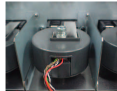
DCCT current sensor (in the PW3337)
