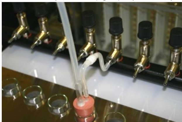
Fig 18. Connection of the cultivation vessel to the main gas dispenser tube.
