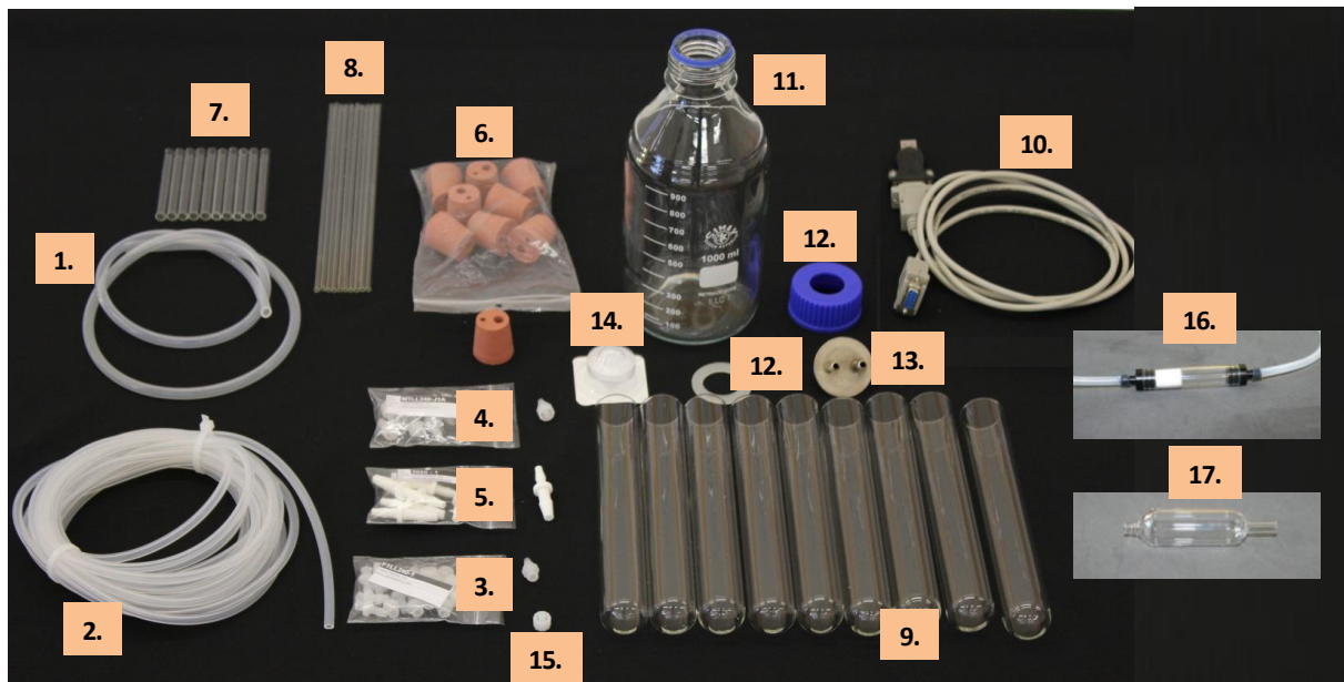
Fig 12: MC 1000-OD kit components delivered with the standard package. The labeling corresponds to the number in Table 1.
