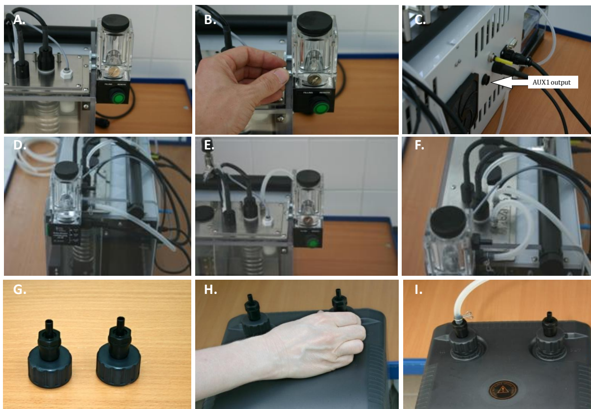
Fig. 7 A,B) Attachment of AC-90 water pump to MC 1000. C) Connection of AC-90 water pump into the AUX1 output. D, E) Connection of water circulation hose to the AC-90 water pump and MC-1000 cooling spiral. F) Connection of MC-1000 cooling spiral with the HC-130A water chiller. G, H) Installation of two port reductions to the top of HC-130A. I) Connection of the cooling spiral hose with the water chiller.
