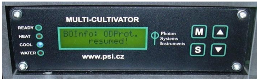
Fig. 26 Control unit display after OD protocol was resumed following MC 1000-OD power outage.
