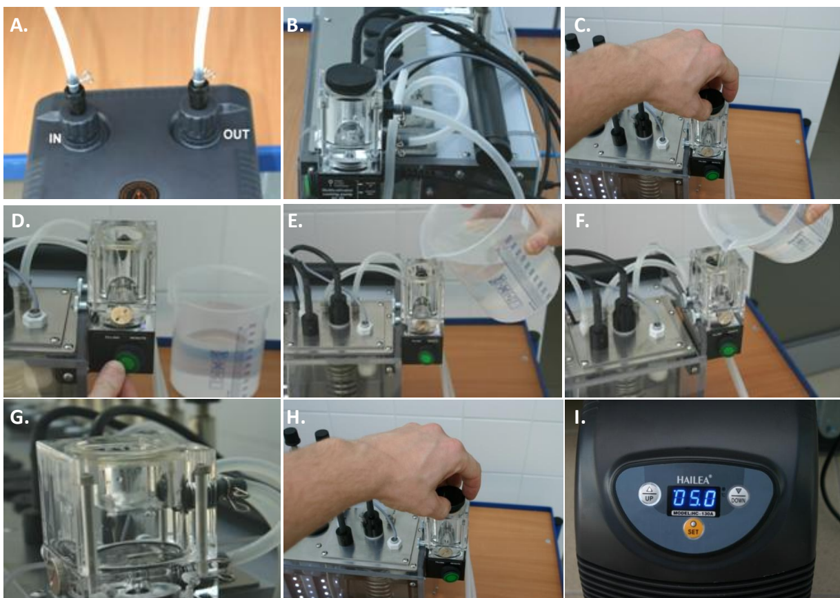
Fig. 8 A,B) Connection of the HC-130A water chiller with the MC 1000. C-H) Description of individual steps for filling of the water pump with the deionised water. I) Setting up the target temperature on the water chiller to 5°C.
