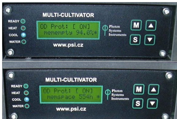
Fig 20. Control unit display with remaining memory space in % and in hours is shown.
