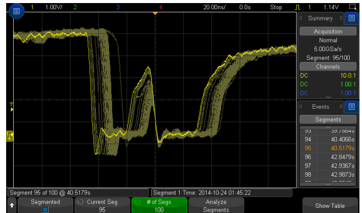
Figure 13a. Screen showing an overlay of all 100 segments for worst case waveform analysis.
