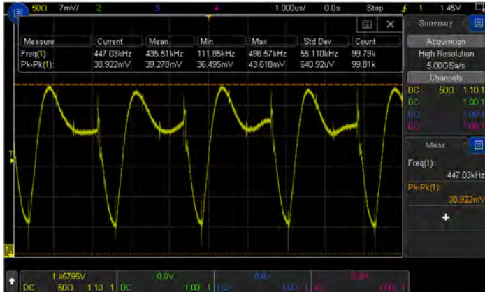
Figure 31a. 3000T X-Series and N7020A acquire not only the power rail ripples but the high frequency transients as well.
