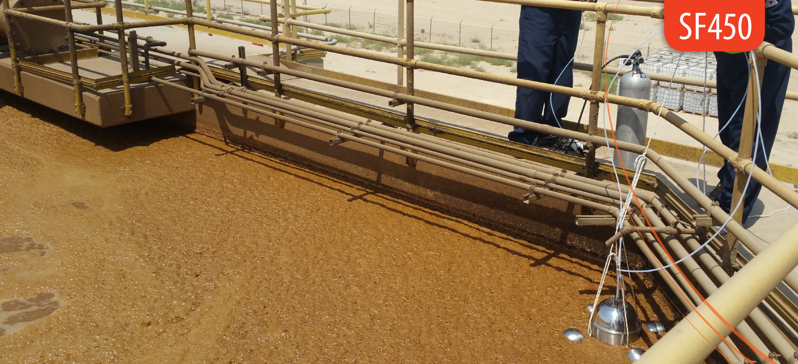
Flux Chamber designed for both solid and liquid surface sample collections.
