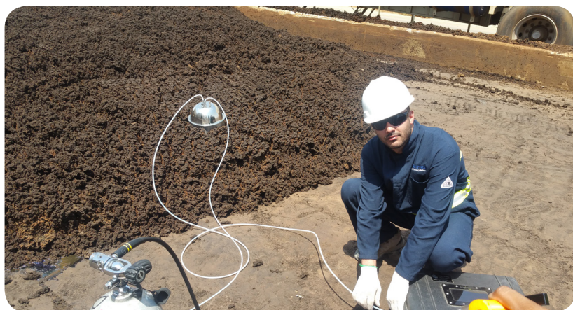
Flux Chamber designed for both solid and liquid surface sample collections.
