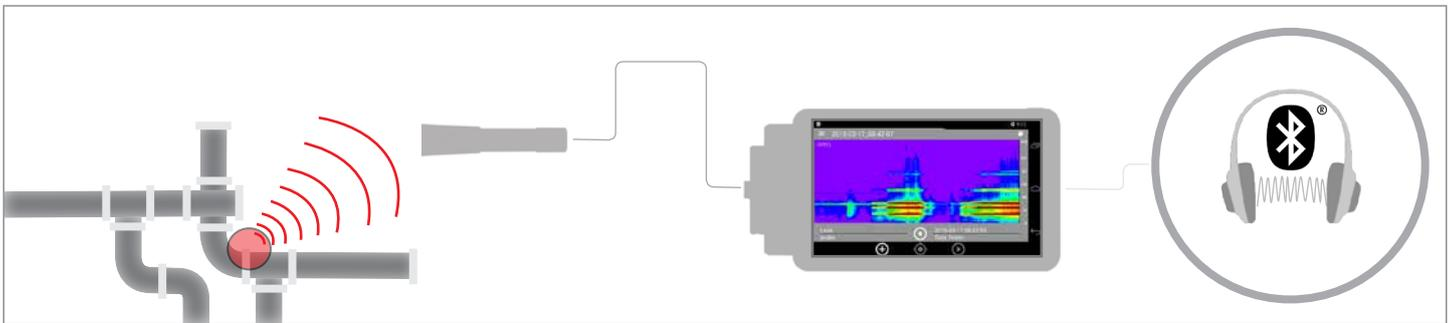
With the **SONAPHONE** you can see and hear everything that happens in the ultrasonic frequency range from 20 to 100 kHz. Thus the innovative sensors pave the way for new domains of use. While other ultrasonic testing devices can only find leaks, **SONAPHONE** can also be used to classify the leak size at the same time. Based on methods of aeroacoustics
