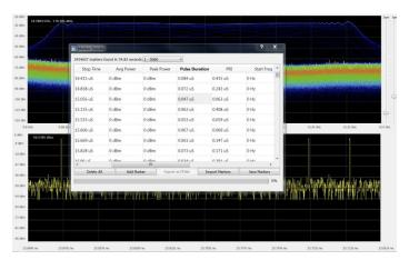
DataVu-PC pulse option provides fast marking of pulses and measurements on large data sets. Above, the results of a pulse search are presented with the pulse measurements of start/stop time, average/peak power, pulse duration, Pulse Repetition Interval (PRI) and start/stop frequencies on up to 2,000,000 pulses. Pulse results can be exported in PDW format for use by other tools.
