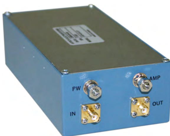
Module style of instrument. The DC power & ground terminals are on the rear face.
