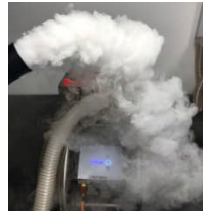
Dense Fog To Visualize Airflow
