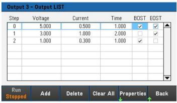
Figure 8. Output sequencing and Output LIST mode setting
