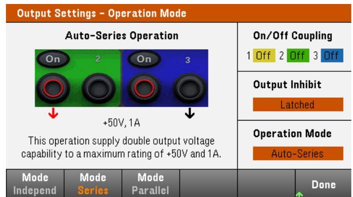
Figure 2. Auto-series operation to double the output voltage
