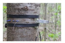
The DC3 has the same layout as the DC2. Only the sensor measuring range is greater than with the DC2. This meets the measurement requirements of fast-growing trees.
