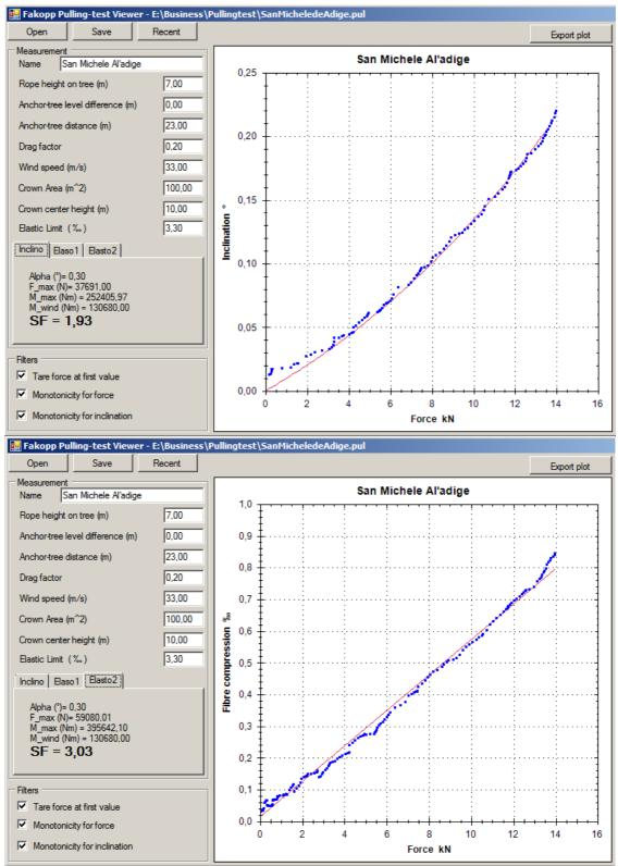
You can toggle between the inclinometer and the two extensiometer curves using the tabs underneath the test parameters. The program automatically fits the appropriate tangential function and straight trendlines on the inclination and deformation data, respectively. It also calculates the statistical parameters and the Safety Factor based on each measurement.
