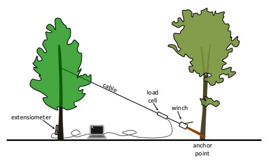
Trunk safety evaluation is a technique very similar to uprooting safety evaluation, except, in this case, instead of inclination, we measure the deformation of the tree trunk. During the pulling test, the trunk bends. Bending causes both compaction and elongation in the trunk, on the side nearest to and farthest from the cable, respectively. By measuring the extent of this deformation on either or both sides, it is possible to predict the safety of the tree against trunk damage.
