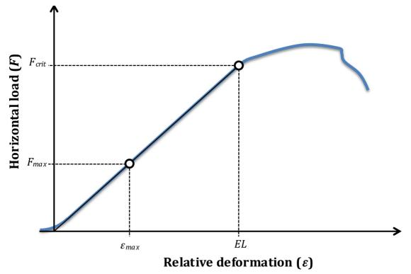
The linear elastic limit is a constant that depends on tree species (see the table at the end of the page). Like in the case of the uprooting test, the deformation induced by the pulling test ( $\varepsilon_{max}$ ) stays well below the *EL*. Based on the measured horizontal load and deformation data, it is possible to extrapolate to the critical load ( $F_{crit}$ ) that would be required to reach the *EL*.
