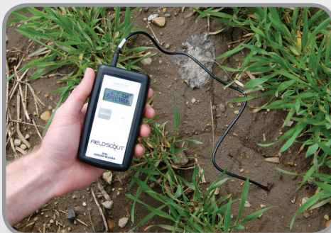
FieldScout Soil Sensor Reader connected to a buried WaterScout SM 100 Soil Moisture Sensor.
