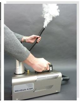
The MiniColt 4S has been designed for air flow testing, visualization tests and particle recovery work. It is a completely portable unit and has the ability to produce anything from a small wisp of artificial smoke to a large plume, on and off power.
