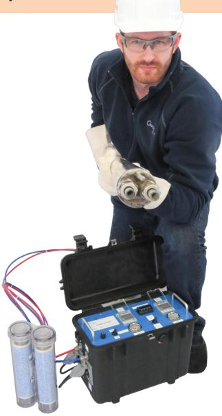
The **dryer unit** is an indicator based Drierite dryer. These appear blue in color while still active, and fade to a pink color when spent. Dryer material is able to be regenerated.
