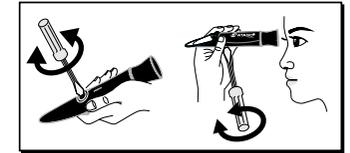
**Note** Don't turn the scale adjustment screw excessively, otherwise, it may cause the refractometer to malfunction. All ATAGO Hand-held Refractometers are delivered after being adjusted in ATAGO factory.
