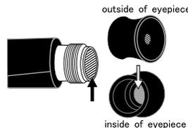
**Note** The instrument is water-resistant rated (JIS-C0920 5th grade jet proof type, IEC specification 529, IP65), however the eyepiece section is not water-resistant.
