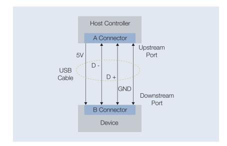
A twisted differential pair Data+ (D+ green wire) and Data- (D- white wire) wires are used for bidirectional communications using half-duplex differential signaling controlled by the host. On an oscilloscope the individual signals can be captured using passive or active analog probes, as well as digital logic probes.
