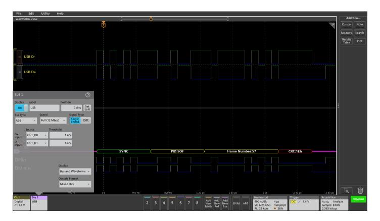
This case shows full-speed USB 2.0 traffic between a PC and a USB drive. A logic probe connected to a FlexChannel<sup>®</sup> input is used to capture the signals. Although the oscilloscope can acquire and decode lower-speed USB bus signals using single-ended probing, the signal fidelity and noise immunity is improved by using differential probing, and is a necessity for high-speed USB signals.
